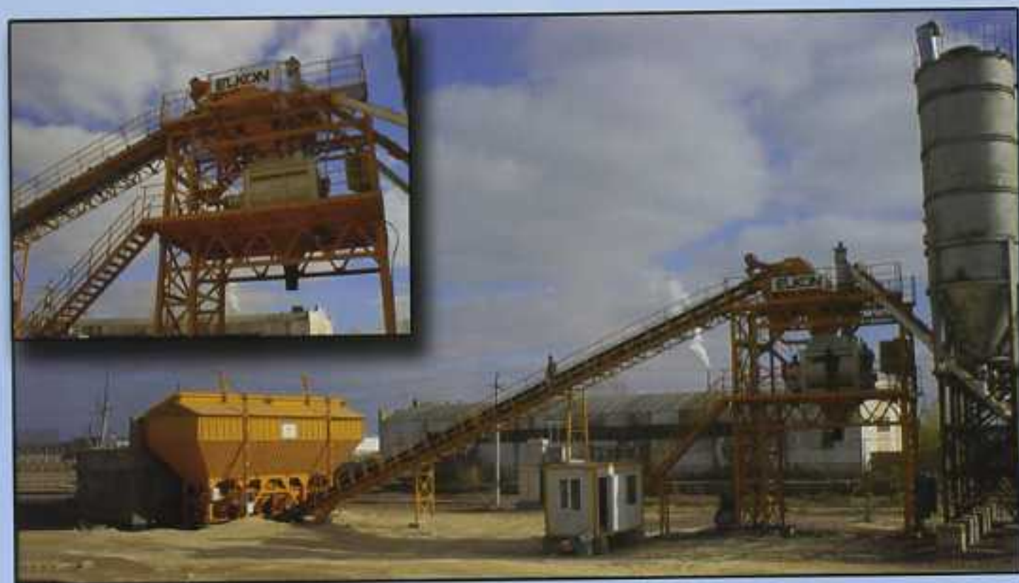
ELKOMIX-120 Fully Automatic Concrete Batching Plant, capacity: 100-105 m 3 /hour vibrated concrete, T type aggregate weight conveyor, transfer belt conveyor, aggregate inline silo 4x30 m 3 , 3000/2000 l twinshaft mixer. (Astana - KAZAKHSTAN)
