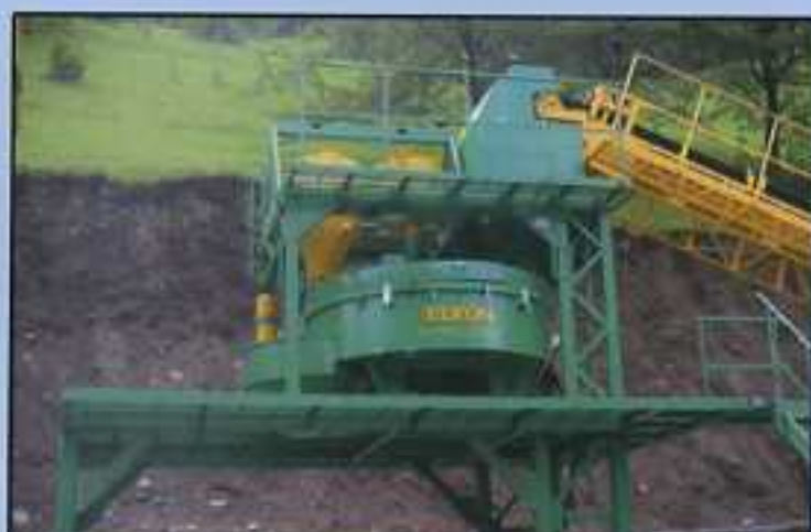
ELKOMIX-60 Fully Automatic Concrete Batching Plant capacity: 60 m 3 /hour vibrated concrete, with aggregate inline silo 4x30 m 3 , transfer belt conveyor, 1500/1000 l pan mixer (1 m 3 vibrated concrete / batch), with aggregate batch silo, with mixer block covering. (Zenica – BOSNIA and HERZEGOVINA)
