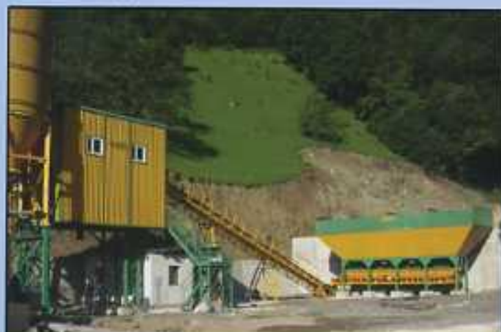
ELKOMIX-60 Fully Automatic Concrete Batching Plant capacity: 60 m 3 /hour vibrated concrete, with aggregate inline silo 4x30 m 3 , transfer belt conveyor, 1500/1000 l pan mixer (1 m 3 vibrated concrete / batch), with aggregate batch silo, with mixer block covering. (Zenica – BOSNIA and HERZEGOVINA)
