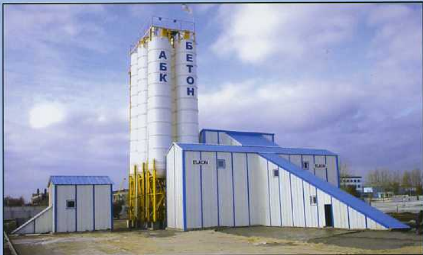
ELKOMIX-6060 Concrete Batching Plant, 1500/1000 l pan mixer (2 units), two independent lines, aggregate inline silo 3x30 m 3 (2 units), heating system, automatic covers above aggregate inline silo, aggregate and cement feeding system from railway, covering, mixer block filter. (Astana – KAZAKHSTAN)
