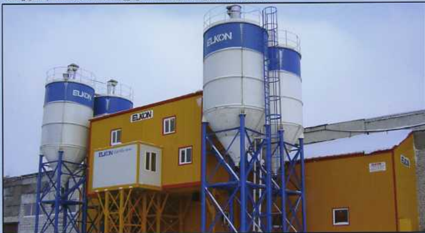
ELKOMIX-6060 Concrete Batching Plant, capacity: 50 + 50 m 3 /hour, two independent lines, loading by skip hoist, aggregate inline silo 2 units 4x30 m 3 , 1500/1000 l pan mixer (2 units), heating system, covering. (Smolensk – RUSSIA)
