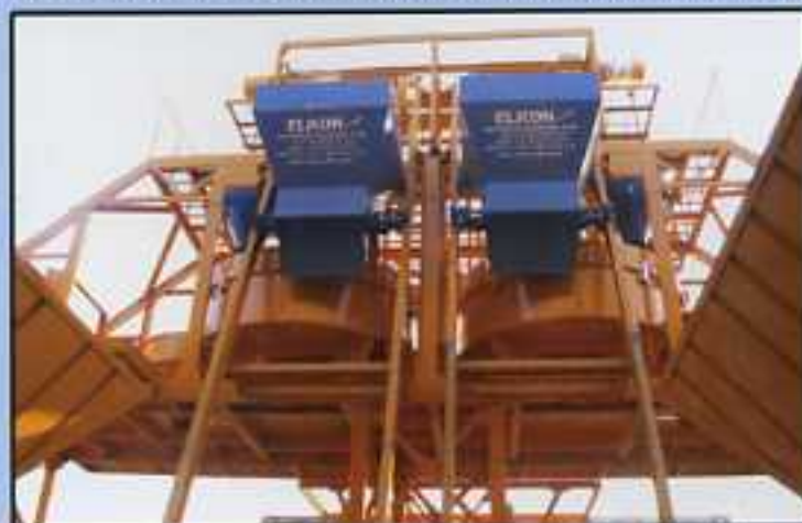
Mixer block of ELKOMIX-6060 Concrete batching plant, with skip hoist, drive system of skip hoists is with two speed motors.
