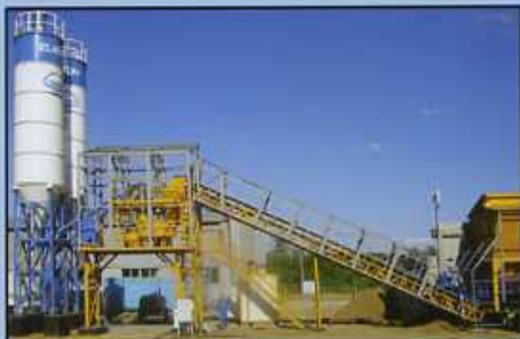
ELKOMIX-35 Concrete Batching Plant, capacity: 30 m 3 /hour with transfer belt conveyor, aggregate inline silo 3x20 m 3 , 750/500 l pan mixer, heating system, automatic covers above aggregate inline silo, covering. (Shuchye – RUSSIA)
