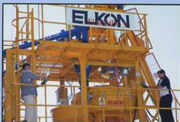
ELKOMIX-35 Fully Automatic Concrete Batching Plant capacity: 30-35 m 3 /hour vibrated concrete, with aggregate inline silo 3x20 m 3 , double speed skip hoist (faster in return), 750/500 l pan mixer (0,5 m 3 vibrated concrete / batch), galvanized water and additive weight batchers. (Sochi – RUSSIA)
