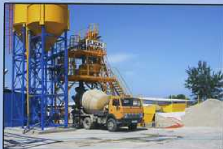
ELKOMIX-35 Fully Automatic Concrete Batching Plant capacity: 30-35 m 3 /hour vibrated concrete, with aggregate inline silo 3x20 m 3 , double speed skip hoist (faster in return), 750/500 l pan mixer (0,5 m 3 vibrated concrete / batch), galvanized water and additive weight batchers. (Sochi – RUSSIA)
