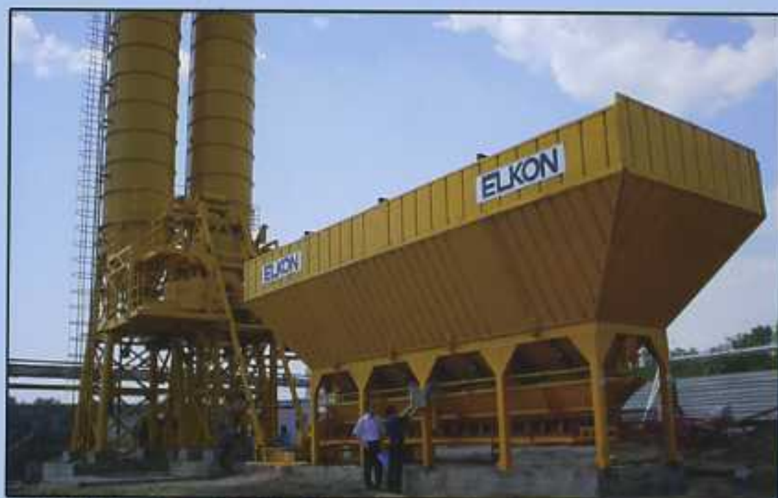
ELKOMIX-6035 Fully Automatic Concrete Batching Plant capacity: 60 m 3 /hour vibrated concrete or 30 m 3 /hour vibrated concrete with two mixers (1500/1000 l planetary mixer, 750/500 l pan mixer) aggregate inline silo 4x30 m 3 , double speed skip hoist (faster in return). (Saratov – RUSSIA)
