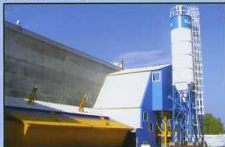
ELKOMIX-6060 Concrete Batching Plant, 1500/1000 l pan mixer (2 units), two independent lines, aggregate inline silo 3x30 m 3 (2 units), heating system, automatic covers above aggregate inline silo, aggregate and cement feeding system from railway, covering, mixer block filter. (Astana – KAZAKHSTAN)
