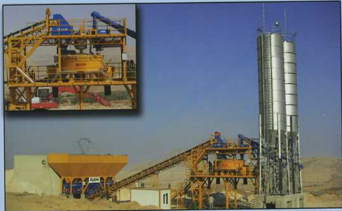
ELKOMIX-120 Fully Automatic Concrete Batching Plant, capacity: 100-105 m 3 /hour vibrated concrete, T type aggregate weight conveyor, transfer belt conveyor, aggregate inline silo 4x30 m 3 , 3000/2000 l pan mixer with two discharge gates. (Damascus - SYRIA)
