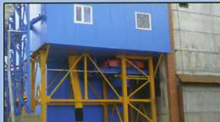
ELKOMIX-60 Concrete Batching Plant, concrete transfer bucket and rail line (45 m), 1500/1000 l pan mixer with double discharging gate, aggregate inline silo 4x20 m 3 , heating system, automatic covers above aggregate inline silo, covering. (St. Petersburg – RUSSIA)
