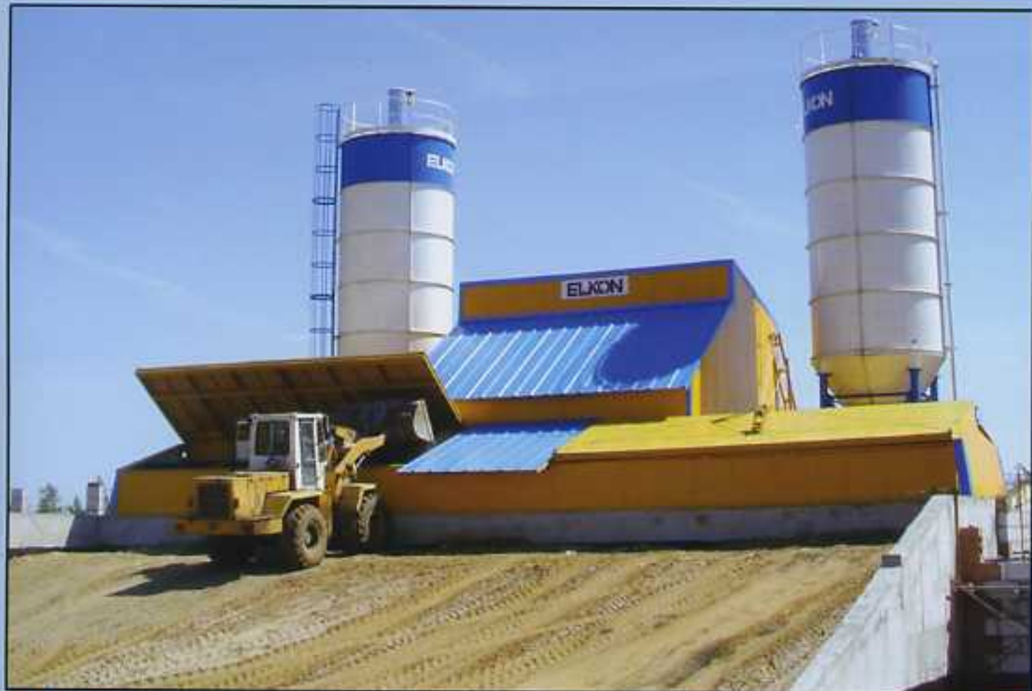
ELKOMIX-3535 Concrete Batching Plant, capacity: 30 + 30 m 3 /hour, two independent lines, loading by skip hoist, aggregate inline silo 2 units 3x20 m 3 , 750/500 l pan mixer (2 units), heating system, automatic covers above aggregate inline silo, mixer block filter, covering. (Minsk - BELARUS)
