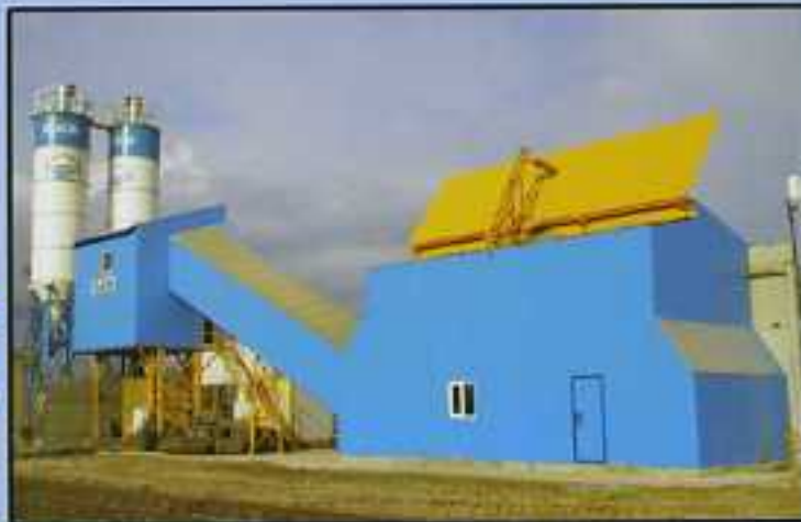
ELKOMIX-35 Concrete Batching Plant, capacity: 30 m 3 /hour with transfer belt conveyor, aggregate inline silo 3x20 m 3 , 750/500 l pan mixer, heating system, automatic covers above aggregate inline silo, covering. (Shuchye – RUSSIA)
